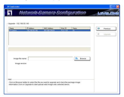
Choose the firmware image file you want to upgrade and press "Upgrade" to start. The device will automatically reboot after upgrade.
